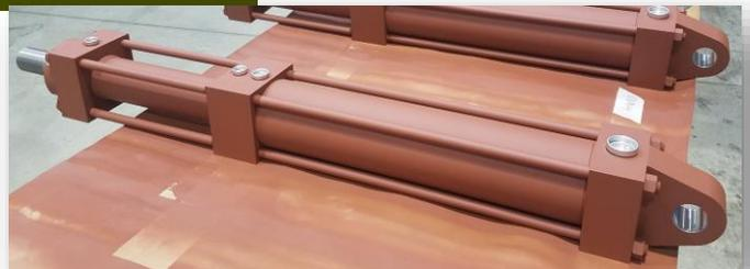
*This Bear-Loc provides nearly 50,000 pounds of fail-safe locking and load holding power.*
