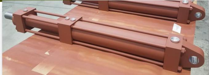
*This Bear-Loc provides nearly 50,000 pounds of fail-safe locking and load holding power.*
