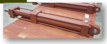
This Bear-Loc provides nearly 50,000 pounds of fail-safe locking and load holding power.
